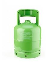
Cylinder - green RAL (6018) - for class 2A refrigerant gas - conforms to Directive 2010/35/EU T-PED - 7 L - handle H 120 mm - base ring D.205 mm - 17E / 25E thread - pressure 36 / 48 bar
